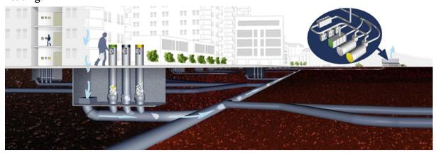
Figure L: Stationary vacuum system in Hammarby.
